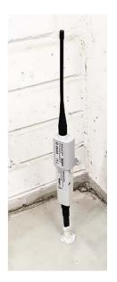
**3.** A plastic hole liner is placed in the bore hole all the way to the bottom. The length of the conduit is measuring depth (max 70 mm) + 20 mm. The minimum length of the conduit can be determined by measuring how much the conduit and the sensor overlap and by adding 10 mm to this measurement. The conduit is cut to the larger measurement.
