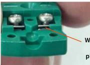
Wires should be secured between the metal plates, not under them.
