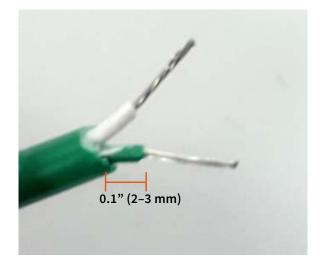
Connect the wires and tighten the screws as shown here. Use white wire for (-) and green wire for (+). Or if the colors are red/ yellow, use red (-) and yellow (+).
