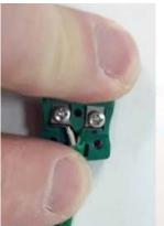
Insulation should extend to the metal connector Outer insulation should fit inside the groove
