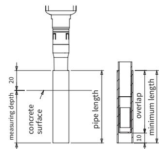
**4.** The seams of the conduit and the casting, as well as the sensor and the conduit are carefully sealed by a layer of Blu-Tack.
